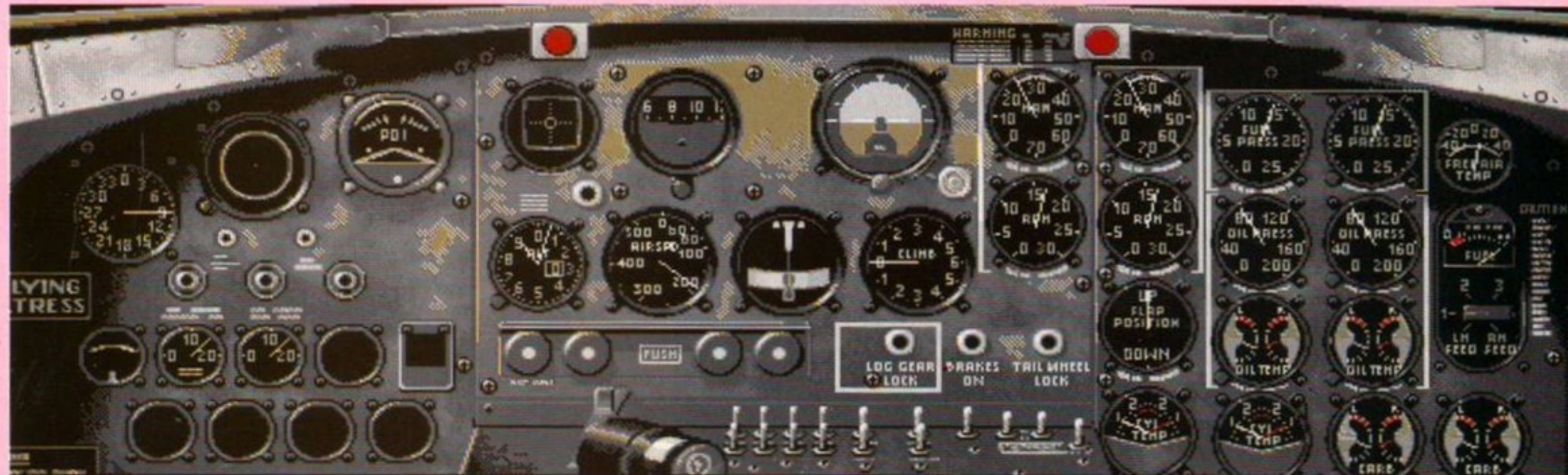
Welcome to the office of a B17 bomber. Most of the dials and controls are not needed for the demo. Central dials worth knowing are; the radio compass (below and right of the leftmost red button); the artificial horizon (to the right of the radio compass); and the altimeter, airspeed indicator, roll indicator and rate of climb/descent (next dial row down).
